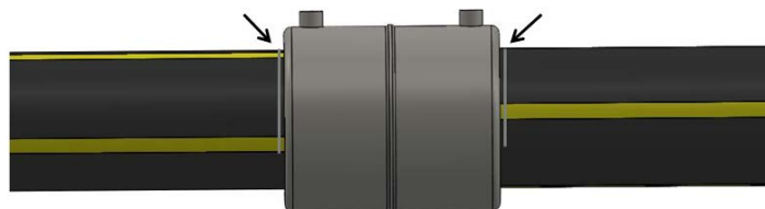
Figure 24: Install fitting to stab depth
